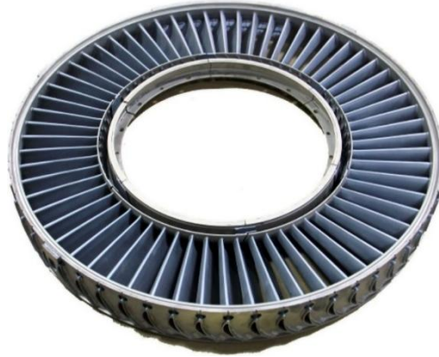
Fig. 5. Brazed aerospace turbine engine components and assemblies, highlighting complex high-performance joints [47].
