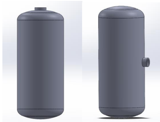
Fig. 2. Concept models of the propellant storage tanks.
